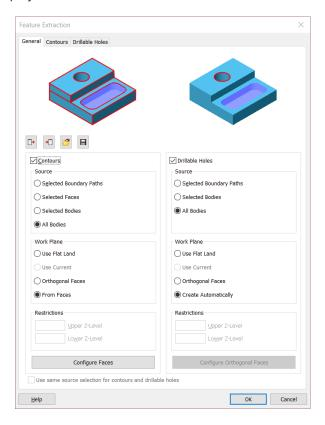
Figure 79 - Feature Extraction options set for multiplane extraction
