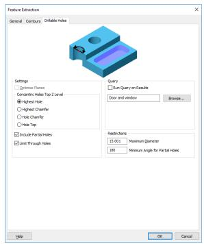
Figure 52 - Drillable Holes tab with Limit Through Holes active
