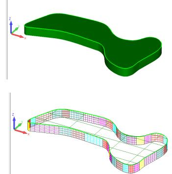
Figure 20 - Extruded surface example in shaded mode
