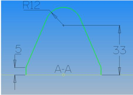
Figure 129 - Geometry set for cross section A-A
