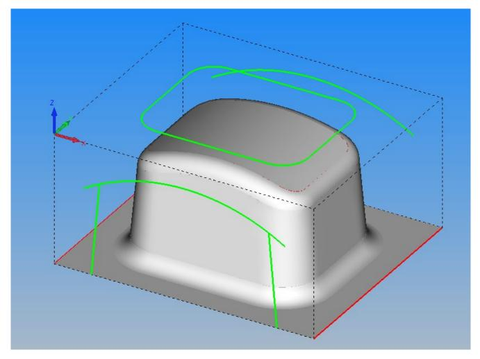
Figure 101 - Completed surface model Example 1 with applied fillets
