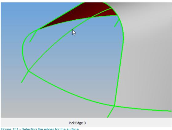
Figure 151 - Selecting the edges for the surface
