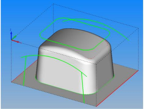
Figure 96 - Surfaces reversed to the correct aspect
