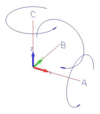
Figure 5 - Left hand rule for axis rotation
