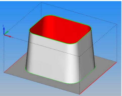
Figure 63 - Completed Ruled Surface
