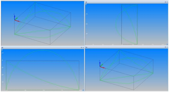
Figure 35 - Coons Patch example drawing
