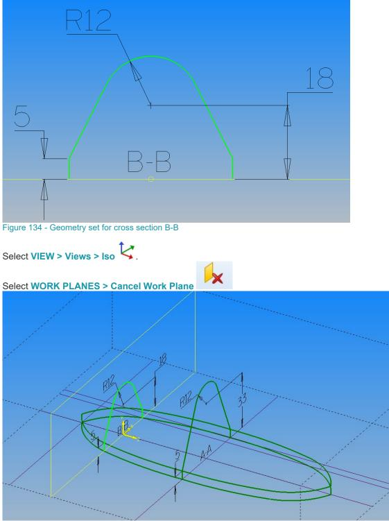
Figure 135 - Created cross section B-B
