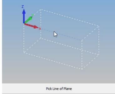
Figure 9 - Selecting a line to Slice Through
