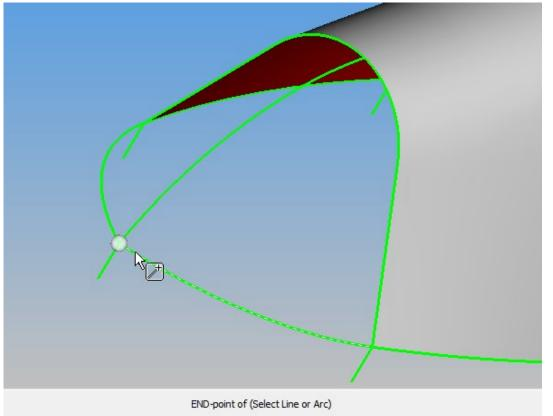
Then using END-point of (F6) <LClick> the end of the 37mm front arc. <RClick> to complete.
