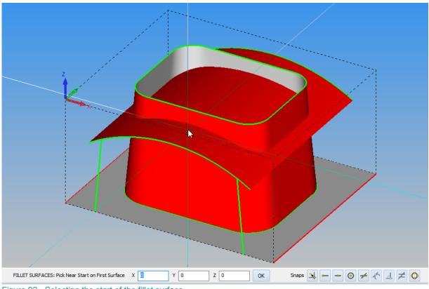
Figure 92 - Selecting the start of the fillet surface
