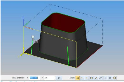
Figure 76 - Second point of the arc
