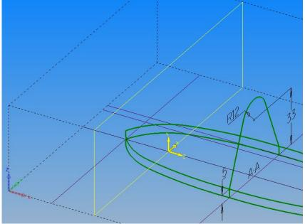
Figure 131 - Work Plane with correct origin location
