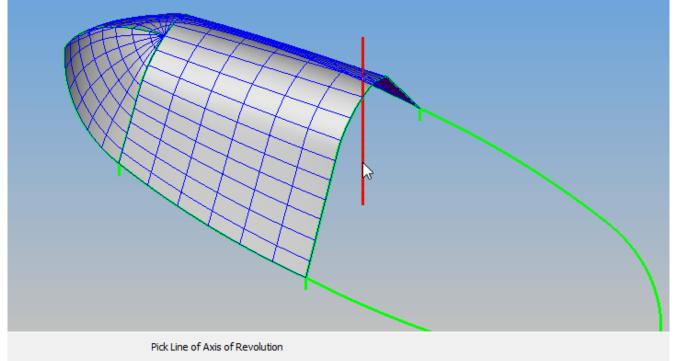
Figure 162 - Selecting the Axis of Revolution
