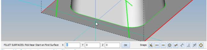
Figure 98 - Selecting the start of the fillet surface
