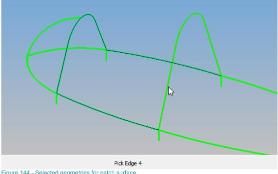
Figure 144 - Selected geometries for patch surface
