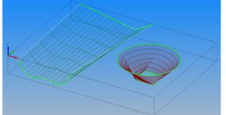
Figure 24 - Ruled surfaces created and viewed in wireframe and shaded
