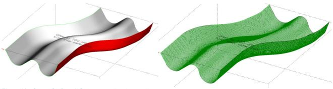
Figure 29 - Swept Surface 2 Curves completed examples
