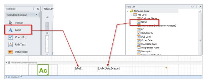
Figure 22 - Assigning a Static Data option and a Dynamic option
